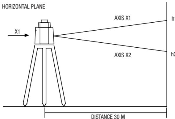
Place the unit about 30 m from a wall as shown in the drawing above. Position the unit with the X1 axis facing the wall.
