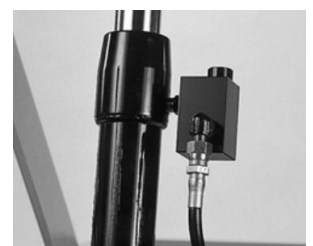
Safety valve in case of overload
