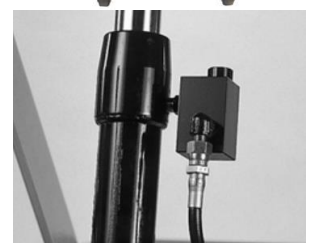
Safety valve in case of overload
